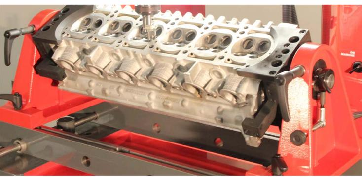
This feature allows a quick and easy mounting of the cylinder head while keeping a powerful clamping thanks to two jaws. It makes easier operations which require the access to different sides of the head.
